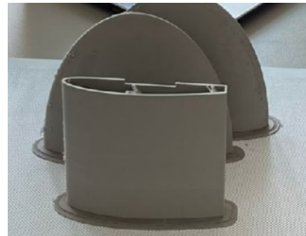
Figure 17. 3D printing of wing sections
