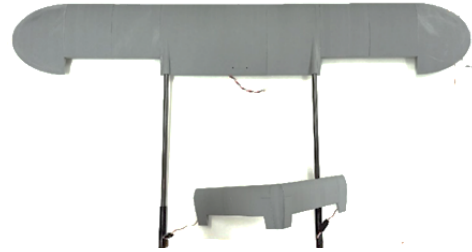
Figure 24. Wing assembly - fixing rods – vertical empennage
