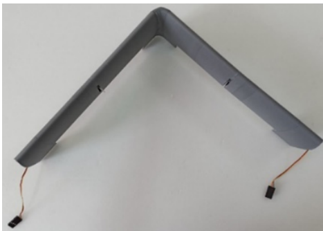
Figure 20. Assembly of the vertical empennage
