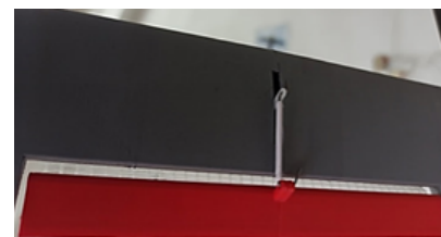
Figure 26. Connecting the rod with the control surfaces
