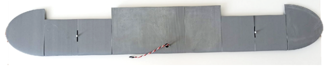
Figure 23. Wing sections positioned on the spar
