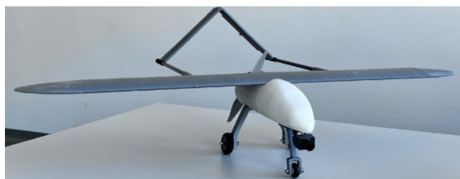
Figure 27. The UAV model manufactured by the FFF process
